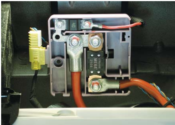
E83 Luggage Compartment Fuse Box w/ Top HiFi Fuse.
